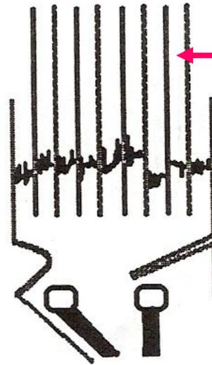
Voltage drop across each baffle extinguishes the arc
